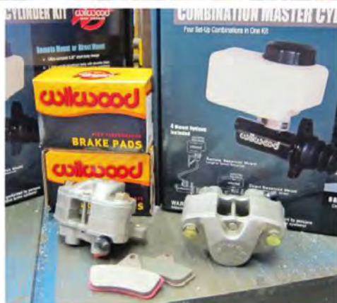
The set of Jr. Dragster brake calipers, pads, and a universal master cylinder kit Wilwood sent us for our brake setup.
