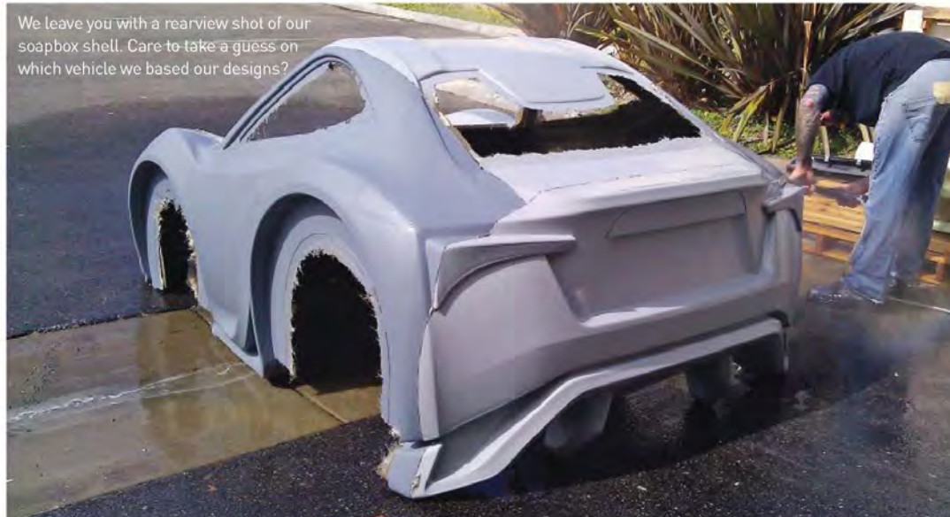
The fiberglass mold of the rearend and roofline of the soapbox.
