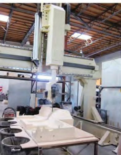
Five Axis shaping the body, using the five-axis mill.
