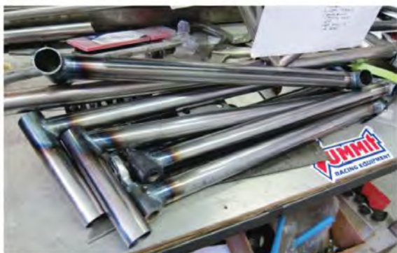
Control arms welded up and ready for fitment.
